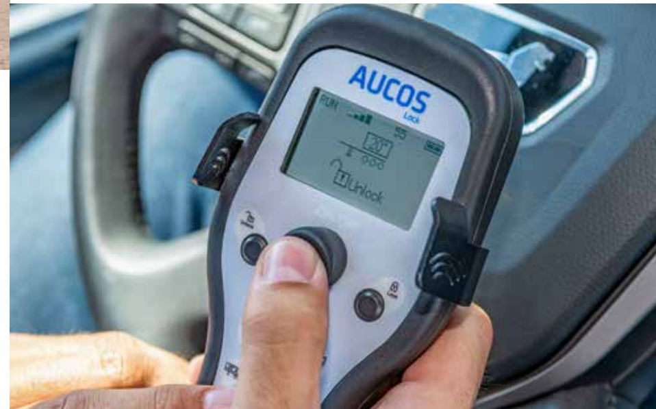
The driver can adjust the container chassis to all containers from 20’ to 45’ at the touch of a button in the cab.
